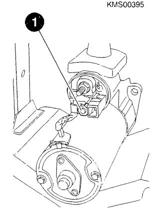
Disassembling solenoid switch
